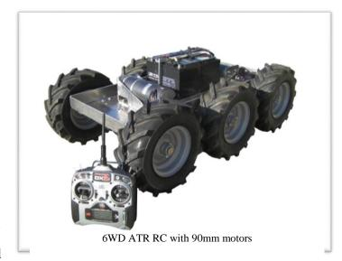
The IG90 ATR frame is 0,35m wide x 0,91m long. The sides are 5 cm high (bottom edge to top surface). As configured with 0,33cm tiller tires shaft and wheel sets it has a ground clearance of about 12,7cm and total width (wheel edge to wheel edge) of about 0,69m. The length of chassis is about 1,04m (wheel edge to wheel edge). The overall height is just the wheel diameter of 33cm.
