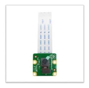
Raspberry Pi Camera Module V2
