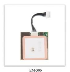
The €35.00 GPS module is another receiver based on the SiRF StarIII chipset. Like the USB GPS dongle described above, the EM-506 provides the position very accurate even in urban canyon and dense foliage environment. The features include a position accuracy of 2.5m, and without any network assistance, it can predict for up to three days the satellite positions.
